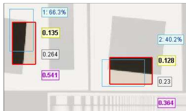
Results of automatic ROI Refinement: Original (cyan) and refined (bold red)
