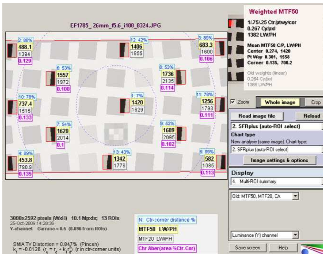
Multi-Region summary plot, showing Center-corner distances, MTF50, MTF20, and Chromatic Aberration (in center-corner %) superimposed on image. Distortion measurements (SMIA TV Distortion, etc.) are shown on the lower-left.
