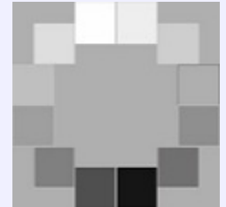
ST-52 ISO-14524 12-patch OECF target
