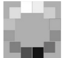
ST-52 ISO-14524 12-patch OECF target
