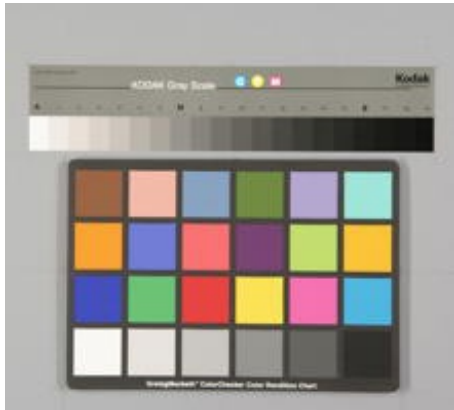
+1 f-stop exposure (first patch saturated)
