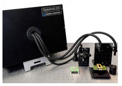
The SpectralLED® Fiber Optic Output configuration provides flexible illumination for applications where space is limited. Systems can be configured with multiple outputs enabling several devices to be simultaneously illuminated at different working locations. Collimating optics are included at the fiber distal end, and custom fiber diameters and lengths are available.
