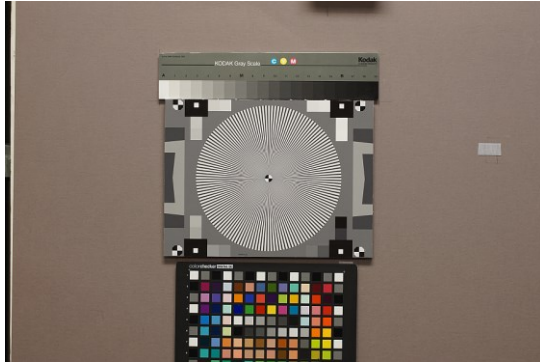
Figure 3. Typical image of Siemens star, scaled to the maximum frequency is slightly above f_{Nyq} .
