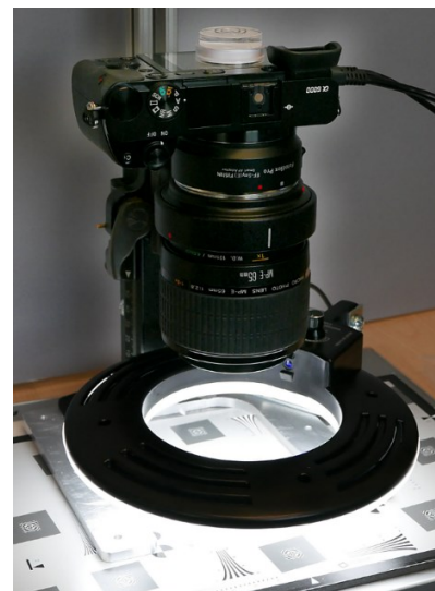
FIGURE 1. CHART MTF MEASUREMENT SETUP
