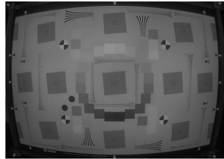
The pixel level in the brightest OECF patch is only 145 — far below the maximum DN for 8-bit files of 255, and gamma = 0.24 is exceptionally low (0.45 is nominal for sRGB color space). The gamma curve is well-behaved, showing few signs of veiling glare or saturation.
