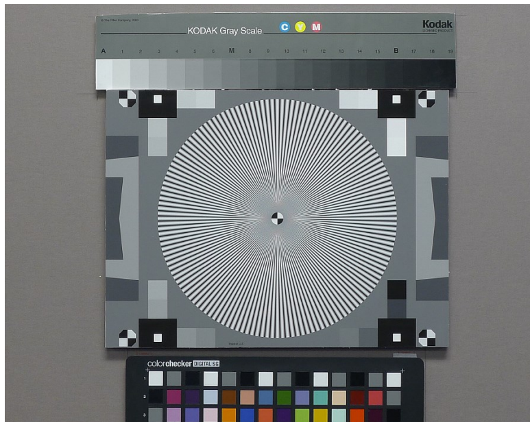
Figure 7. Typical image (cropped) including Siemens star and slanted-edges to the left and right of the star.
