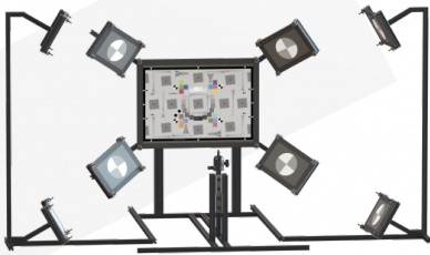
Imatest Ultra Wide Field of View Fixture
