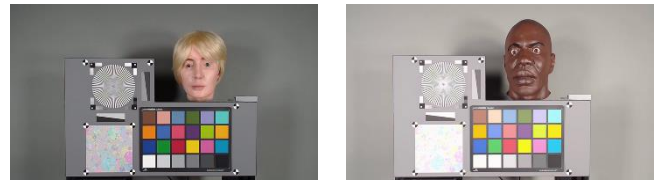
Figure 1. Example VCX test scene; Left: Alexis mannequin; Right: Richard mannequin; Both scenes captured under identical illumination conditions.
