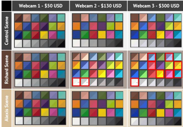
Figure 3. Simulated ColorChecker patches from each scene compare the target patch color against the corresponding average measured patch value. Bolded borders indicate saturation in one or more color channels.
